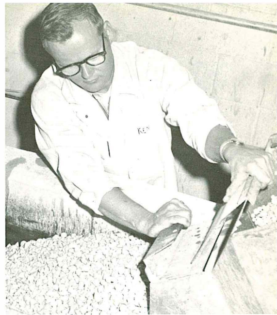
George Krueger, Lorco Lab Technician, adds Wheelabrator media to a vibratory machine
